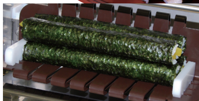
4 hosomaki (small roll) can be set on cutting table : 2,200 rolls / hr
